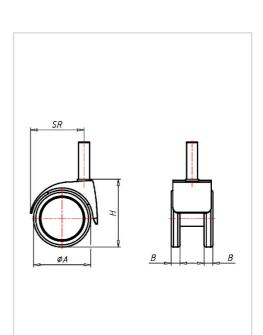
Swivel castorWheel-Ø A x width B mm: 75x13+13Load Capacity kg:60Load capacity tested according to EN 12530 and EN 12527Overall height H mm:93Stern mm:11x30Swivel radius SR mm:71Wheel bearing:Nylon plain bearing
